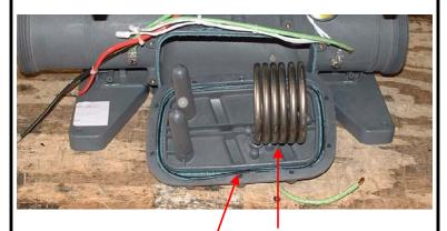
Non-Corrosive Weld Free Heater Housing
